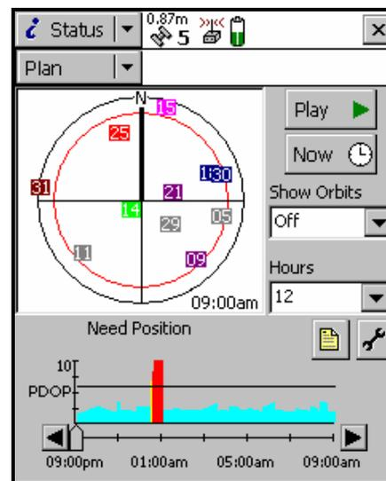
**Figure 5: User interface on a professional receiver showing satellites (above) and PDOP (below).**
